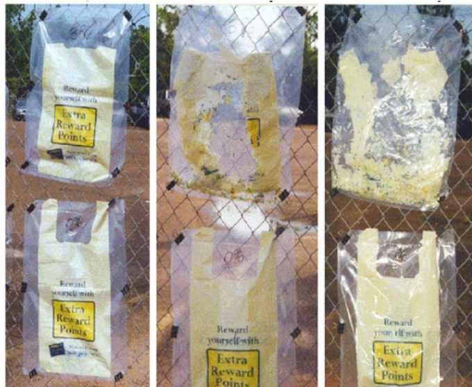
Illustration of photo and thermal degradation of a shopping bag incorporating EPI's TDPA® Additive (top row) vs. a bag without EPI's TDPA™ Additive (bottom row). Test procedures follow ASTM D5272 "Outdoor Exposure Testing of Photo Degradable Plastics" Guidelines.
